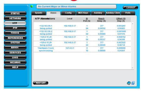
You can see that all time servers have a Reach of 377 and the Hardware Clock is the one the NTP daemon is using for the time.
